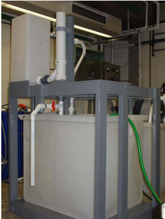
Figure 1: Recirculating Trickling Biofilter Media Testing Module and Its Operational Diagram.
